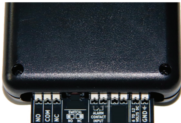
ADM-215 Remote Alarm Delay Connections
